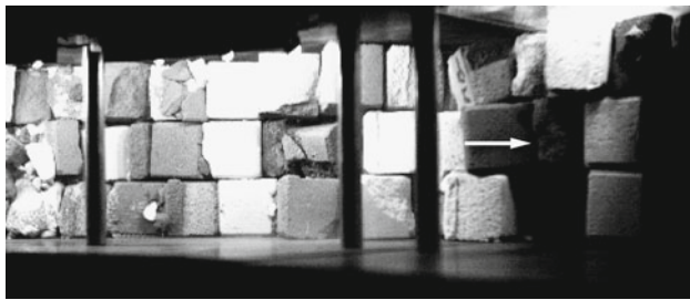
Fig. 7 View into the “A” channel of the model. Image taken by the black and white high speed camera during the experiment. The arrow indicates the flow in the x' -direction and serves as a scale. Its length is 32 mm, which equals the initial side length r_0 of the intact blocks. The rock blocks remain in contact during the entire experiment. This simulation was performed at an angular velocity \omega of the centrifuge of 30.4 rad/s
